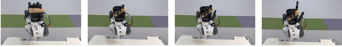
(a) Regrasping via switching grasp type: from thumb-index precision pinch to power grasp
