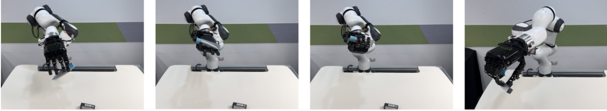
(b) Simultaneous grasping of two objects through shifting the first object along the palm
