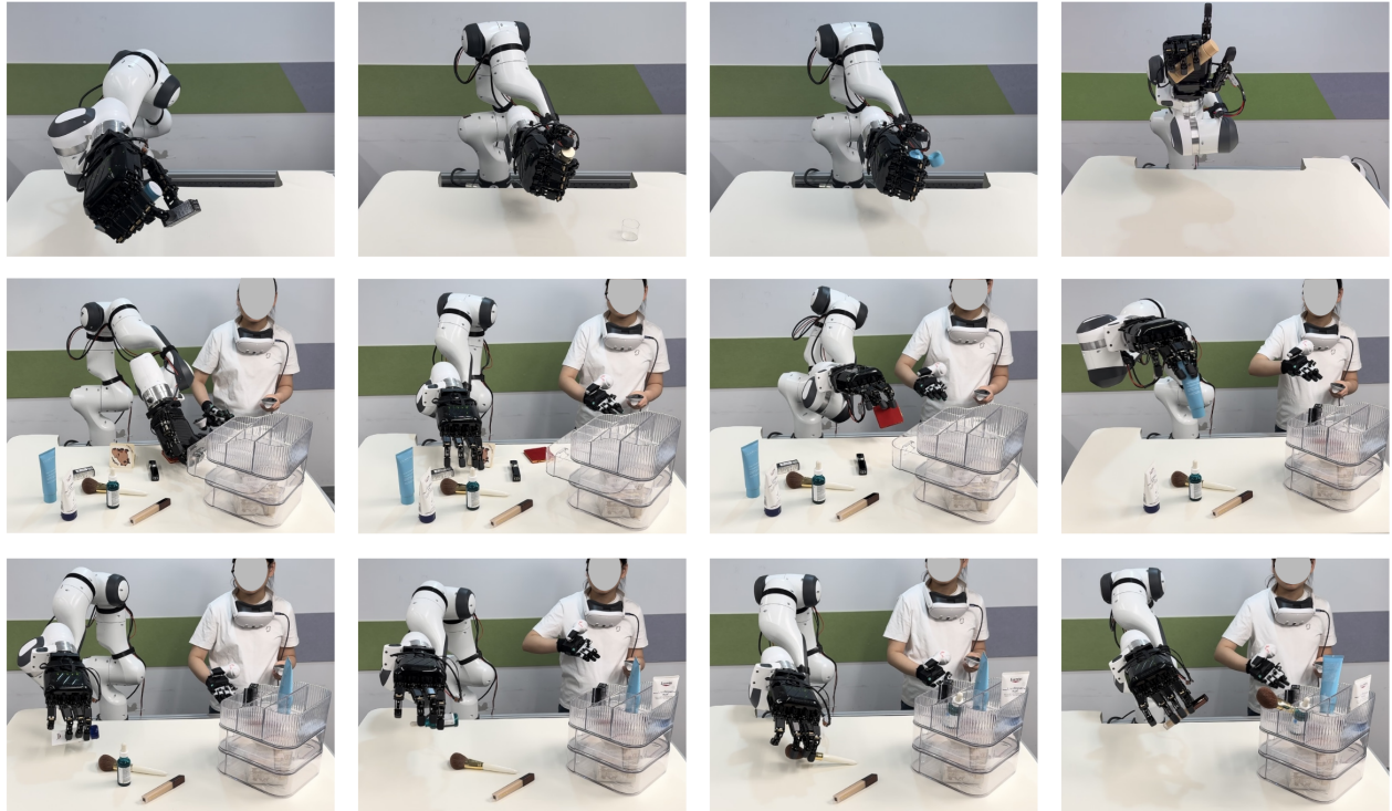
Figure 1 Our hand-arm teleoperation system achieves dexterous in-hand manipulation, including multi-object grasping, rotation, and regrasping. It also successfully manages grasping of various cosmetic items during a long-horizon cluttered-table organization task.
